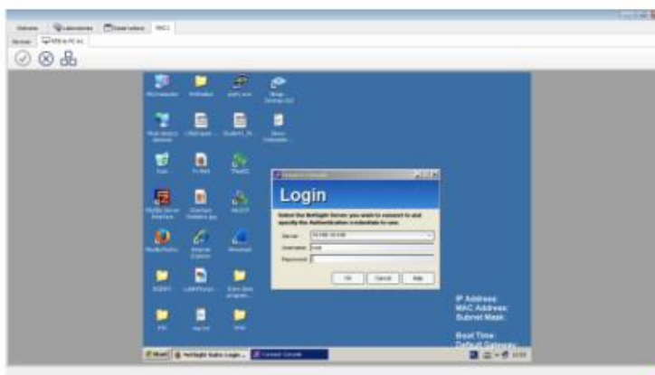
Figure 4 VNC access to a remote virtual PC
